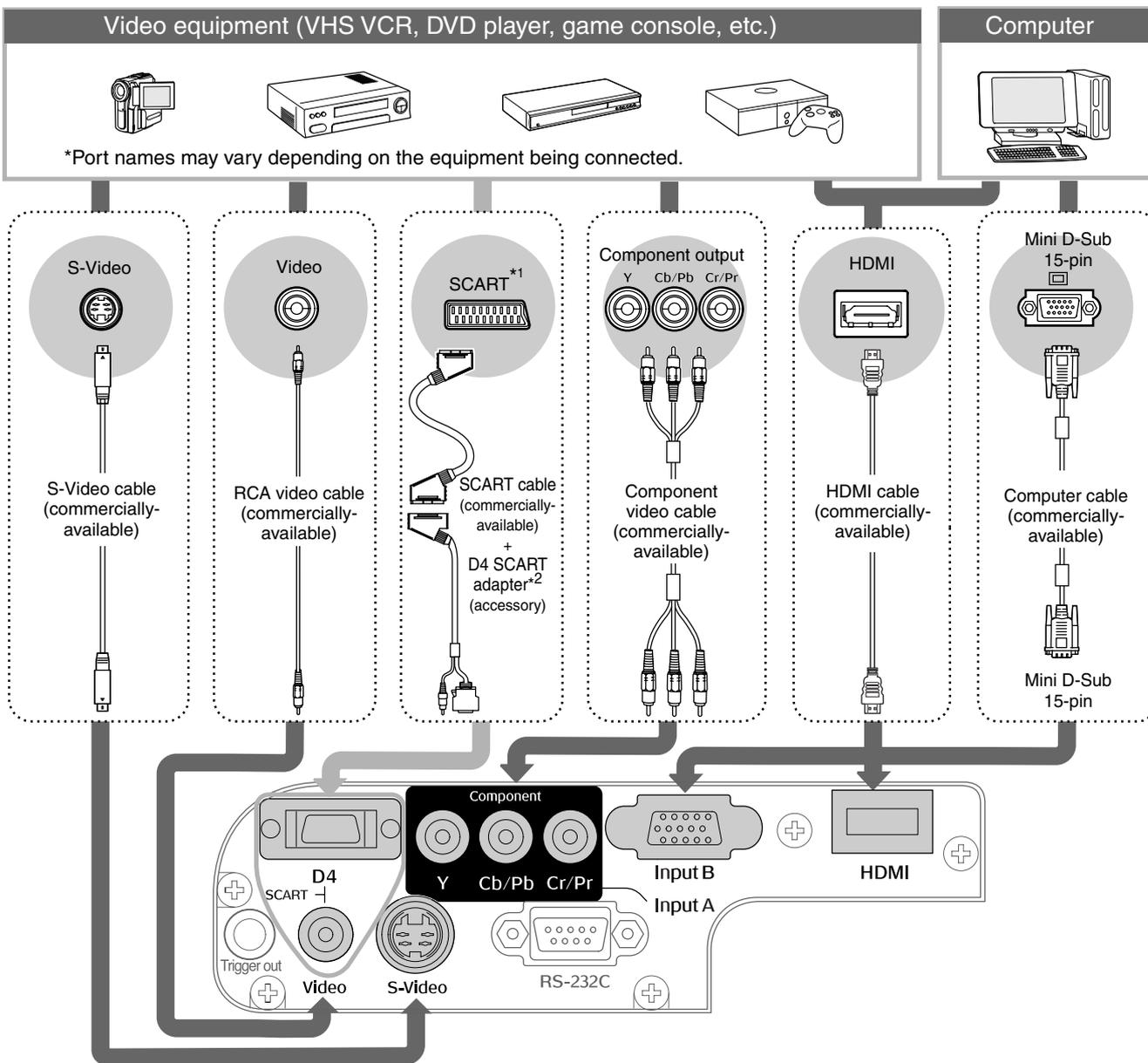
\*1 If a DVD has been connected using a D4 SCART adapter, change the "D4/SCART" setting in the "Input Signal" to "SCART". "Selecting the image source" p.15
