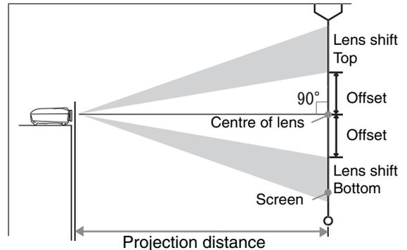
The height from the centre of the lens to the bottom of the screen will vary depending on the lens shift setting.
