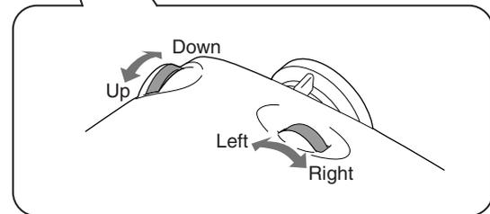
You can shift the image by 100% in the vertical direction, and 50% in the horizontal direction. However, you cannot shift the image to these vertical and horizontal limits simultaneously.
