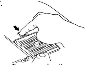
Put your finger under the latch and pull it upward.
