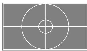
This can be used to check that the projector is not tilted but rather set up parallel to the screen.
