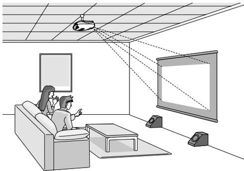
\* Even if projection will be from the screen side, set up the screen and projector so that they are parallel.
